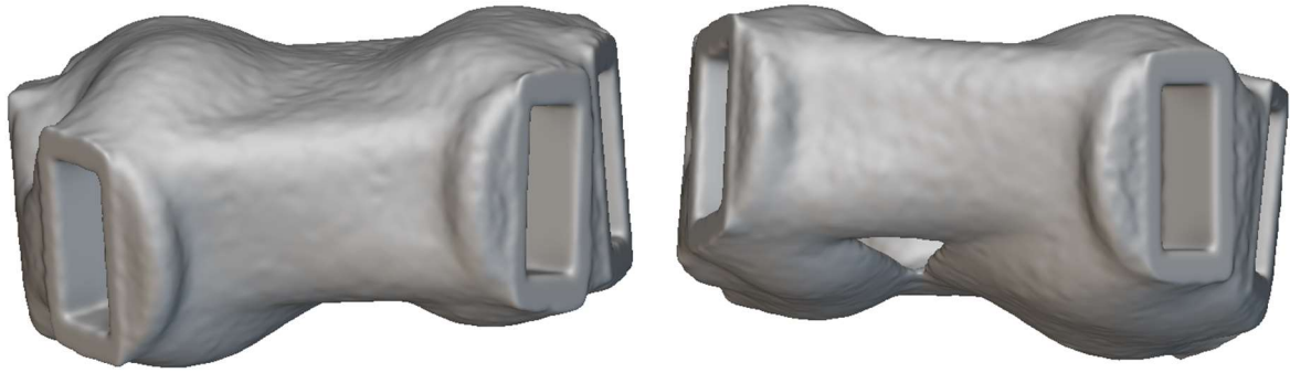
Figure 6.47 - Third attempt: topology optimization of the joint using nTopology
