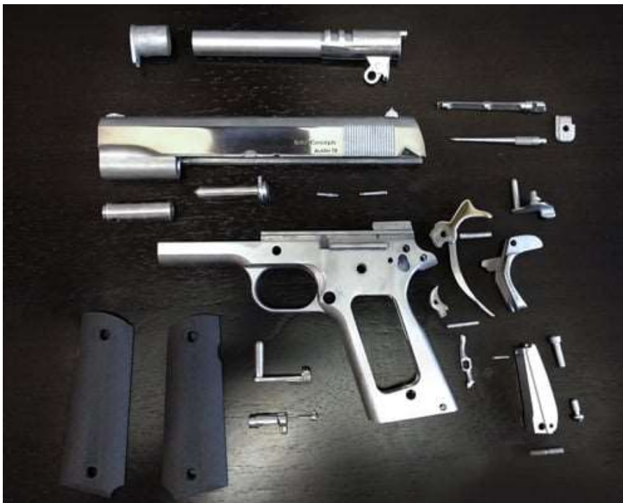
Figure 2.35 - Commercial gun made with additive manufacturing (Milewski, 2017)
