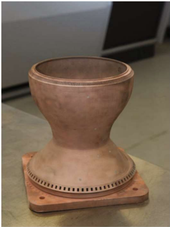
Figure 2.28 - Copper rocket nozzle by NASA (Milewski, 2017)
