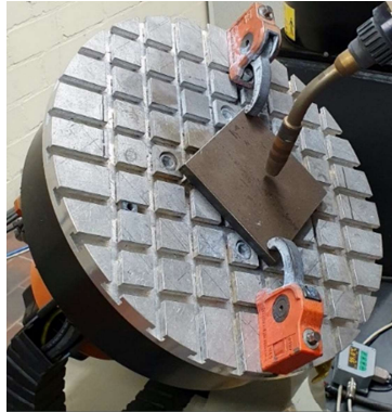
Figure 2.3 - Base plate installation for WAAM
