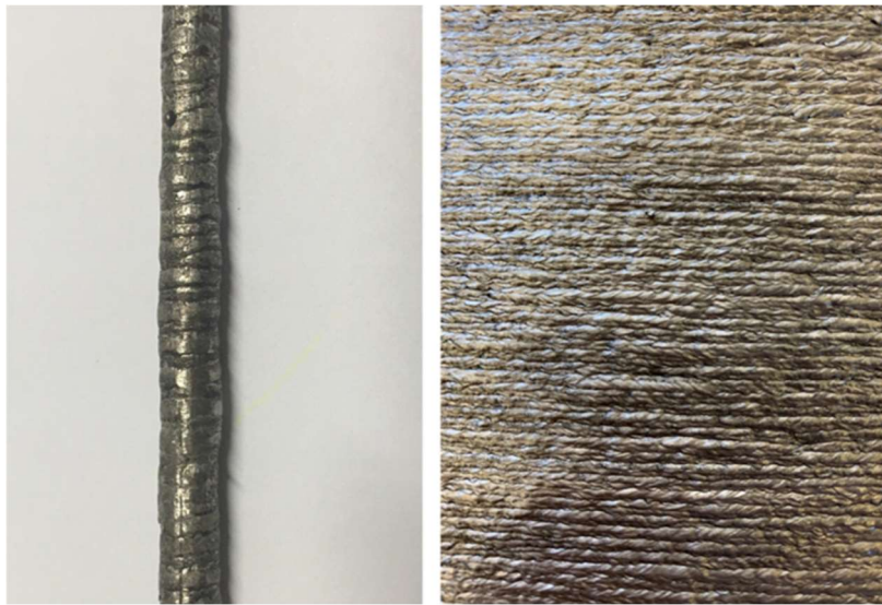
Figure 2.17 - Wire-and-arc additive manufacturing dot-by-dot (left) and layer-by-layer (right) (Vittoria Laghi, 2020)
