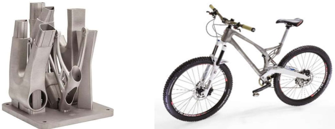
Figure 2.22 - Customized bike frame using metal additive manufacturing (Milewski, 2017)
