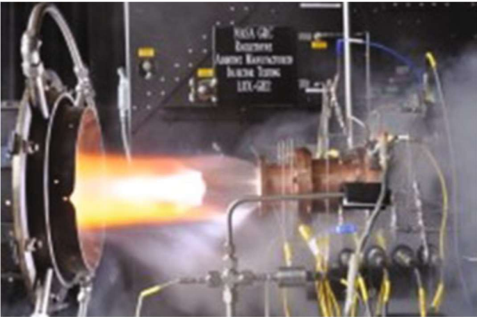
Figure 2.28 - Copper rocket nozzle by NASA (Milewski, 2017)
