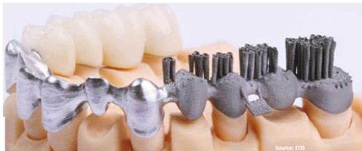
Figure 2.25 - Dental bridge made using metal additive manufacturing (Milewski, 2017)
