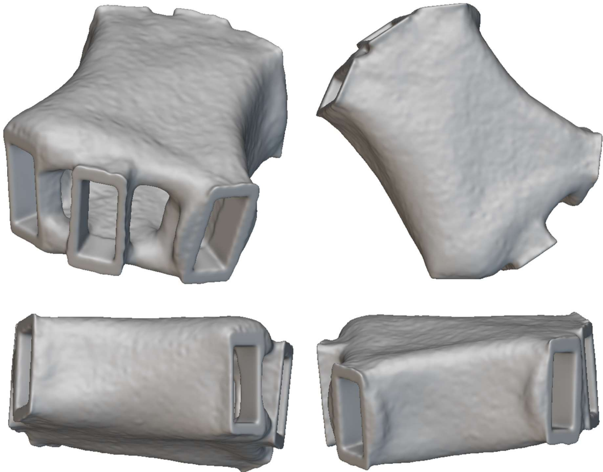
Figure 6.49 - Fourth attempt: topology optimization of the joint using nTopology
