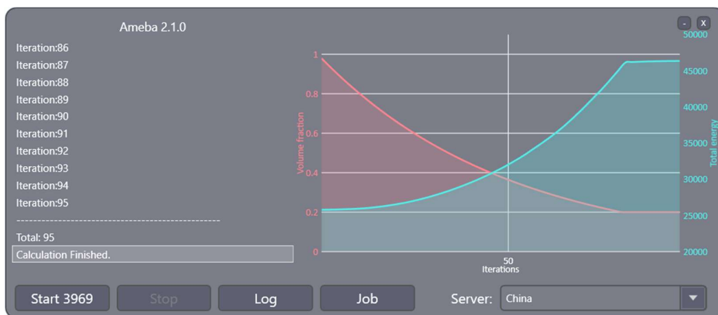
Figure 4.23 - Solver graph in which is possible to watch the volume reduction and the strain energy evolution during the topology optimization process
