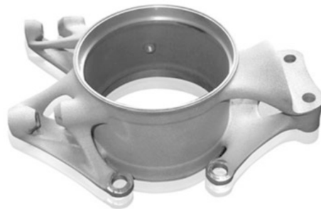
Figure 2.30 - Steering knuckle made with metal additive manufacturing (Milewski, 2017)
