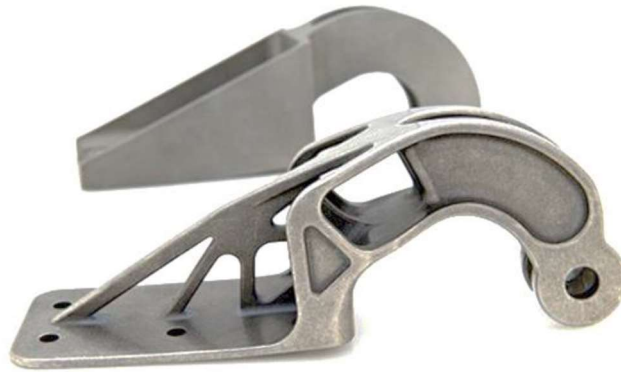
Figure 2.29 - Nacelle hinge bracket of the Airbus A320 (Linden, 2015)
