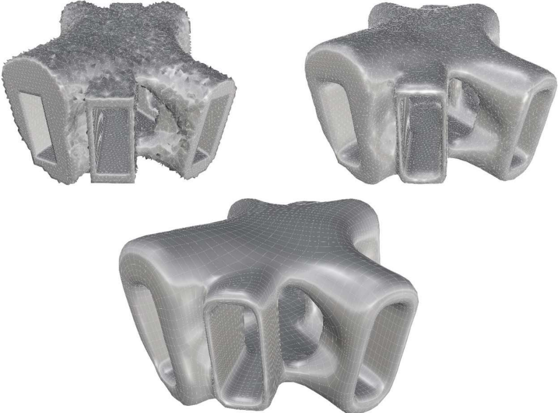
Figure 6.56 - Initial joint geometry (top-left), smooth joint (top-right) and final joint geometry (bottom)
