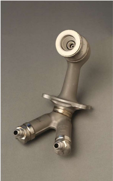
Figure 2.27 - GE Aero LEAP fuel nozzle (Milewski, 2017)
