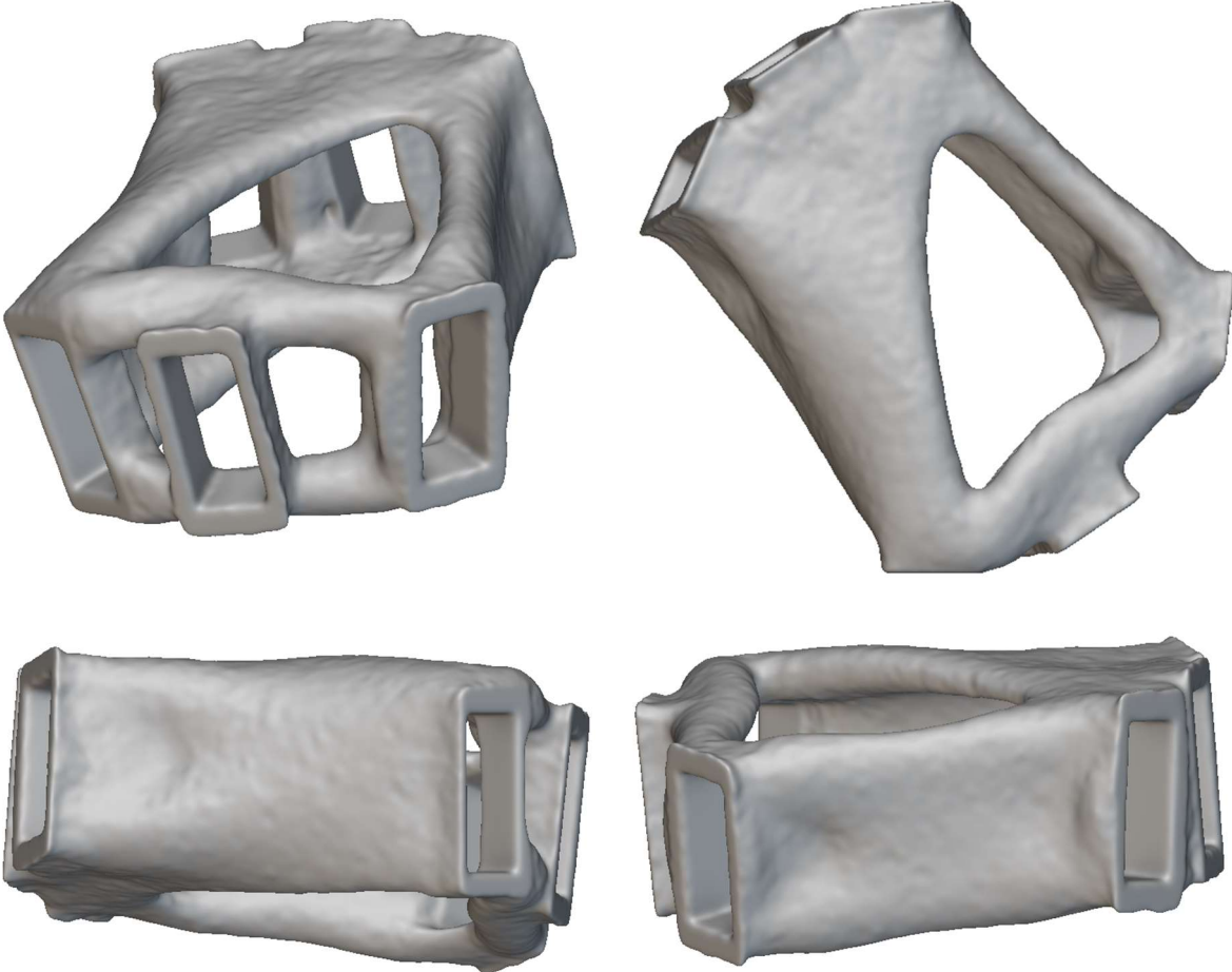
Figure 6.51 - Fifth attempt: topology optimization of the joint using nTopology
