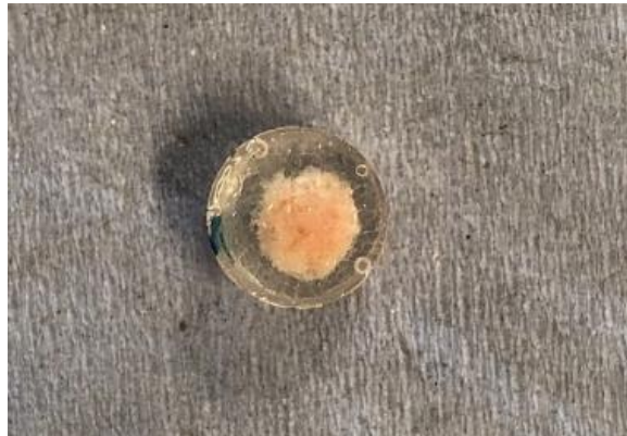
Figure 12: bone specimen embedded in epoxy resin.
