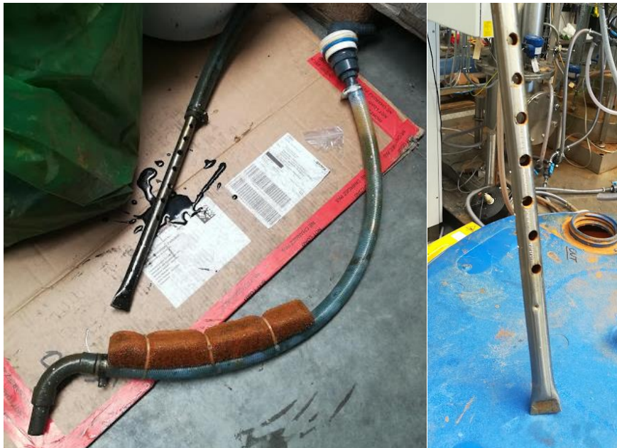
Figure 4.8: system for radial inflow (right picture) and floating outflow pipes in the sedimentation barrel
