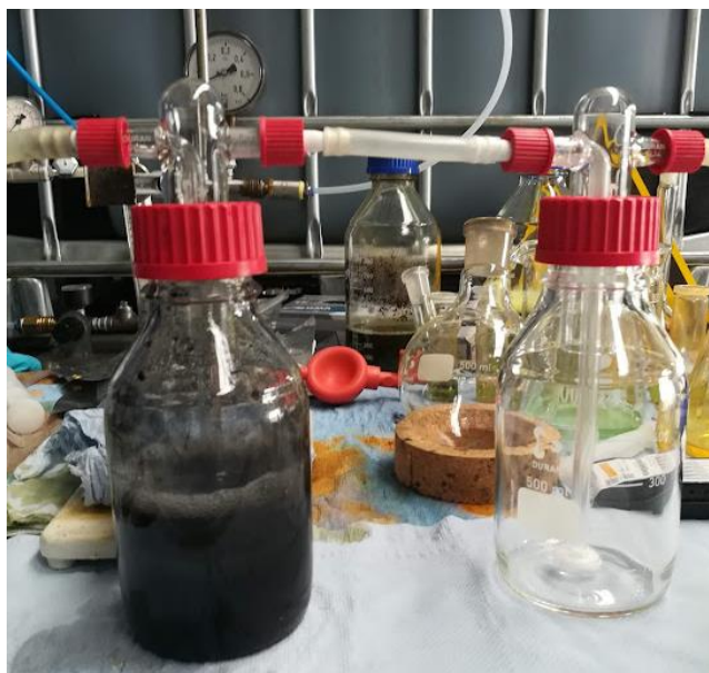
Figure 4.15 The doubling system of gas washer and the dark solid particle formation of FeS
