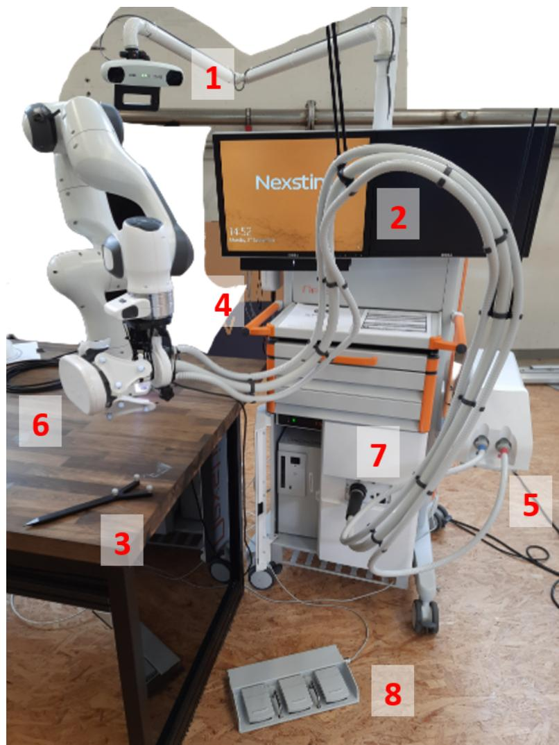
Figure 3.1: The Nexstim NBS cart: 1) Tracking unit; 2) monitors; 3) digitizing pen; 4) EMG amplifier; 5) cooling unit; 6) cooled coil; 7) TMS Stimulator; 8) pedals.
