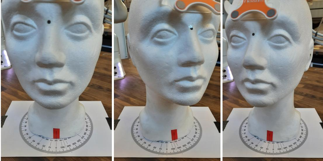
Figure 7.5: The three head poses for the head compensation approach experiments; 0 degrees (left), +20 degrees (middle), -10 degrees (right).
