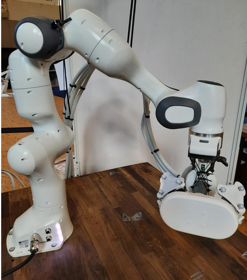
Figure 6.4: Panda robot equipped with the last connector version; the coil is fasten with cable ties to the connector base.
