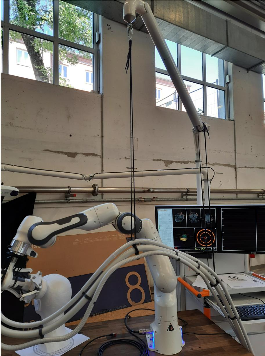
Figure 6.2: Support laces for cables and cooling tubes.
