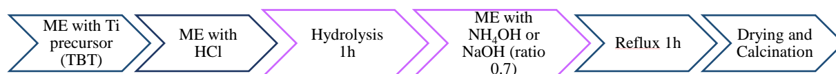
Figure 4.2.1-A. Operative scheme for the synthesis of titania with the neutralization approach when HCl is used. The hydrolysis and reflux time are 1 hour; both NH 4 OH and NaOH are tested.
