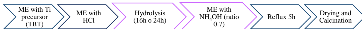
Figure 4.2.1-B. Operative scheme for the synthesis of titania with the neutralization approach when HCl is used. The hydrolysis is 16 or 24 hours and the reflux is 5 hours in both cases; NH 4 OH is only used.
