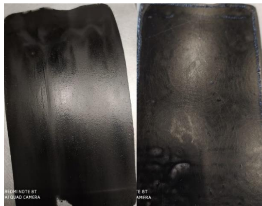
Fig.23 Micrometric knife deposition of teflon base (left) and formulation n°1 (right)
