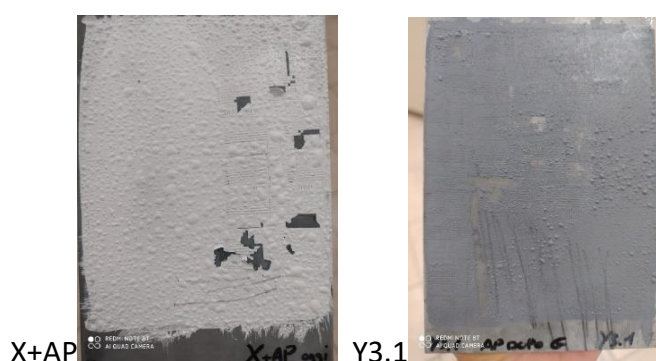
Fig.46 Deposition X+AP (acrylic base) and Y3.1 after water immersion test
