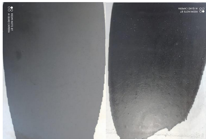
Fig.24 Mayer bar deposition of teflon base (left) and formulation n°1 (right)
