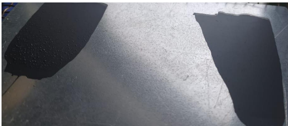
Fig.22 Micrometric knife deposition of teflon base treated with TRM (right) and not treated with TRM (left)
