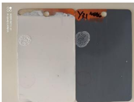
Fig.51 Acrylic base (left) and Y3.1 (right) after drop by drop resistance test
