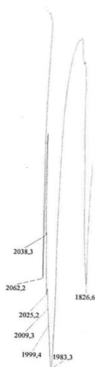
Figure 29: IR spectrum of the products of the reaction between [\text{Rh}_7(\text{CO})_{16}]^{3-} and \text{Au}(\text{Et}_2\text{S})\text{Cl} in DMF, under CO atmosphere.
