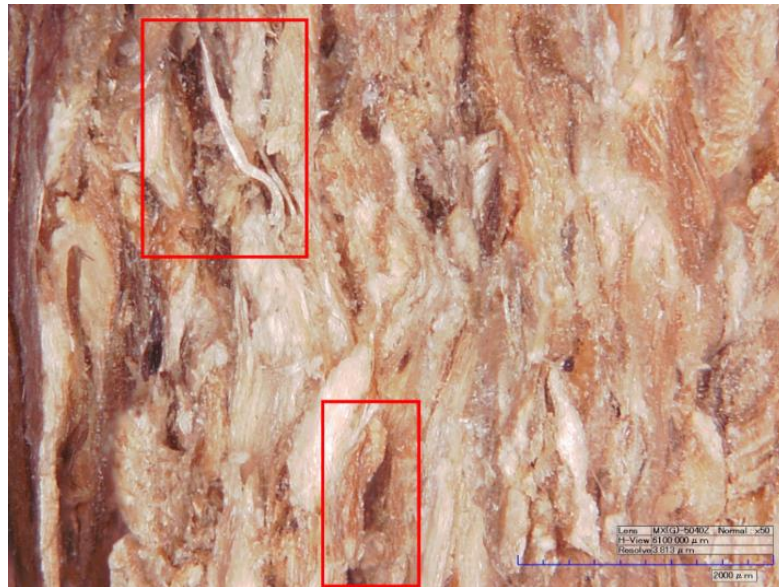
Figure 2.4.10 Optical microscope's image of panel with 10%/dry w of activated SPI
