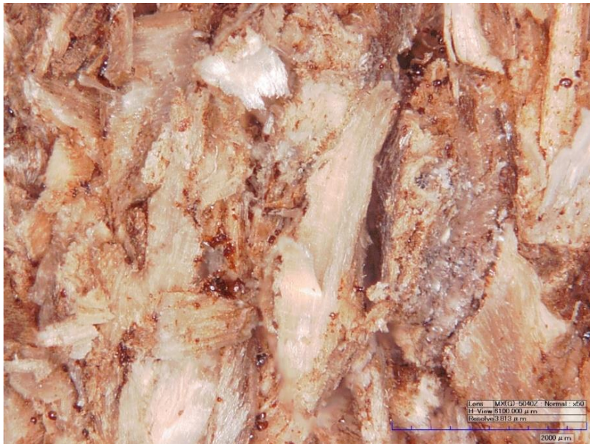
Figure 2.3.2 Image at optical microscope of sample made with normal HS and lignin UPM (10%/dry w.)
