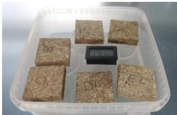
Figure 2.2.3 Experimental set-up for samples' exposure to 99,9% humid environment
