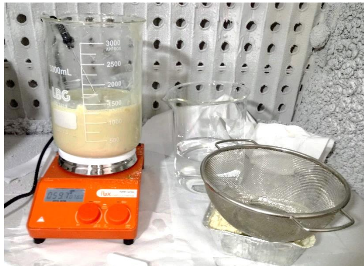
Figure 2.2.2 Experimental setting for basic hydrolysis of SPI
