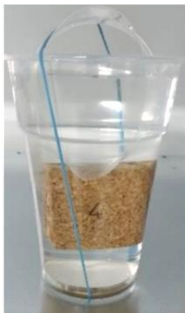
Figure 2.2.4 Experimental set-up for 24 hours of immersion in water
