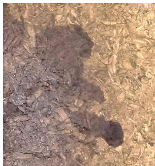
Figure 2.4.8 Darker spots on tile produced with 10%/dry weight on activated WPI
