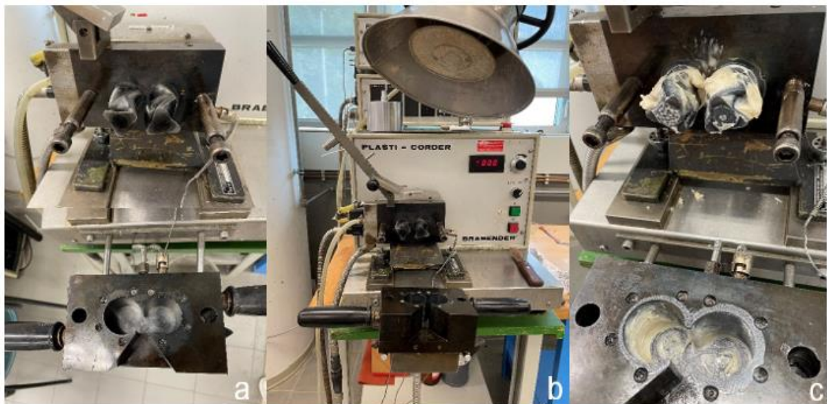
Figura 12: Camera e viti del BraBender Plasti-corder (a), strumento BraBender (b), viti e camera post mescolamento (c)
