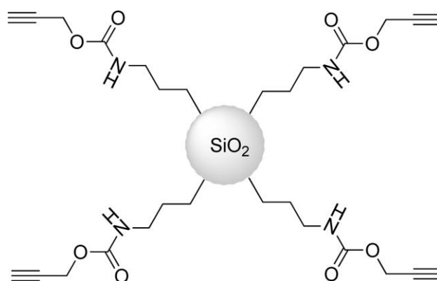
Fig. 1.1: Alkyne-modified silica nanoparticle (SiO 2 @Yne). 3
