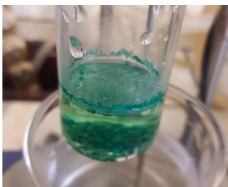
Fig. 2.27: Synthesis in DMF/H 2 O 3:1 of the new Cu-MOF, after 168 hours, before the work-up.
