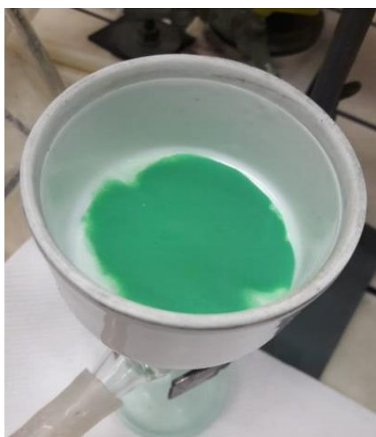
Fig. 2.26: The product of the MOF synthesis in 2-propanol after the washing with 2-propanol.
