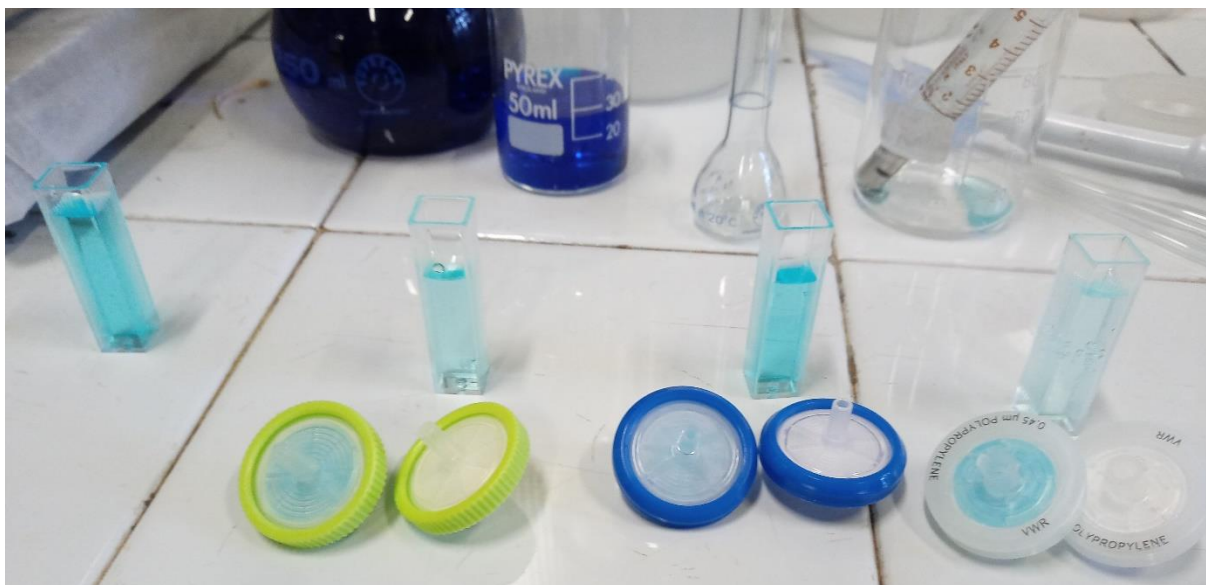
Fig. 5.4: A 4 ppm solution of MB (cuvette on the left) was filtered with (from left to right): PES filter (green), Nylon (polyamide) filter (blue) and Polypropylene filter (white). The recovery values are respectively 78%, 14% and 55%.
