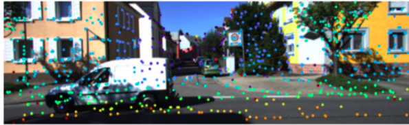
Figure 4.9: The sparse depth maps used were generated by using all the mapped points, falling inside the camera frustum, without taking into account possible occlusions. This leads to particularly relevant mistakes in the case of moving objects.
