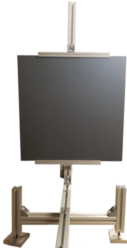
Figure 2.3: Planar reflective target mounted on a sliding carriage.
