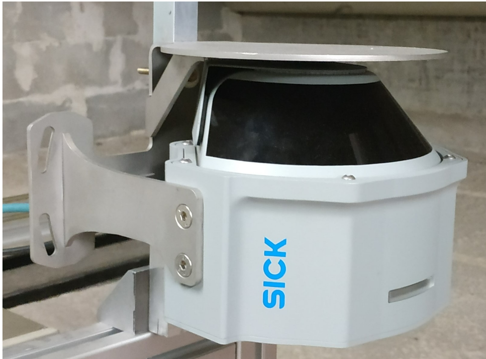
Figure 2.1: Instrument under test (SICK MRS6000) mounted on its bracket.
