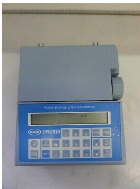
Fig. 16 Spectrophotometer used for the analyses described in the following paragraphs 3.2.1
