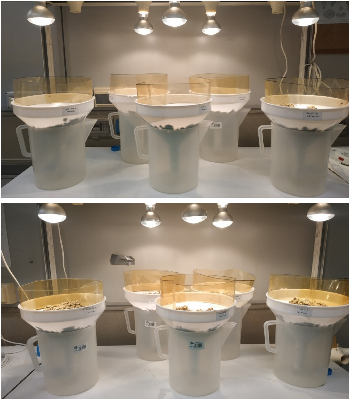
Fig. 21 Representation of the Berlese funnels used for the experiment. Photos (a) replicates from 1 to 5, photos (b) replicates from 6 to 10
