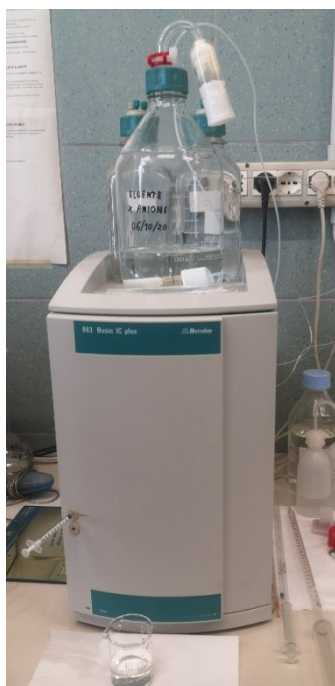
Fig. 20 Ion chromatograph (Metrohm IC 883 Basic plus) used for the determination of soluble forms of nitrogen
