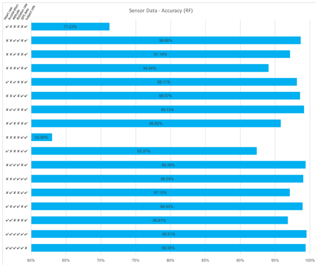
Figure 6.7: Accuracy scores of various sensor data configurations for random forest. A checkmark indicates that the sensor data was included.
