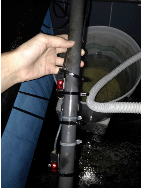
Figure 1. Photocells attached to a PVC tube were then loaded inside the tanks.
