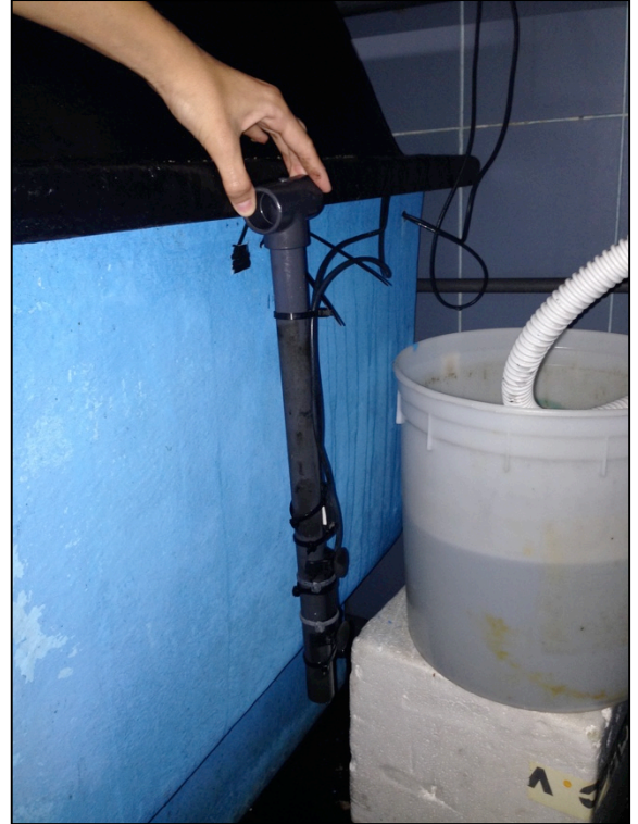
Figure 2. Example of how photocells were positioned inside the tanks in vertical position.
