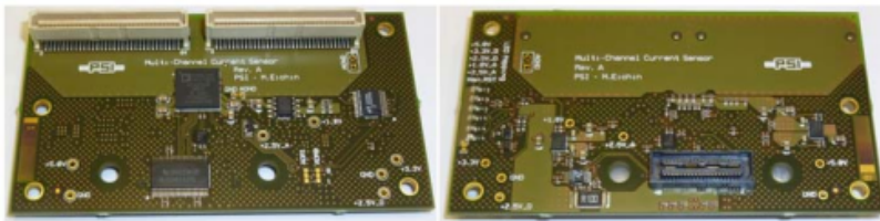
Figure 29: Picture of the two MCCS boards equipped with the ADAS1128 chips.
