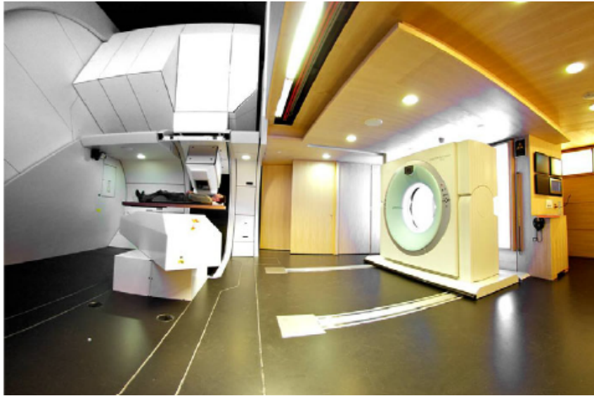
Figure 19: Gantry 2 treatment room layout showing the isocentric design and fixed floor setup, together with the in-room CT.
