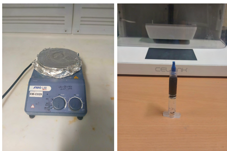
(a) Hot plate used to stir and heat the various inks (b) syringe used to load the ink into the BIO X printer
