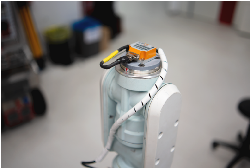
FIGURE 4.1: Picture of the IMU mounted on the PA10 robotic arm in the laboratory.
