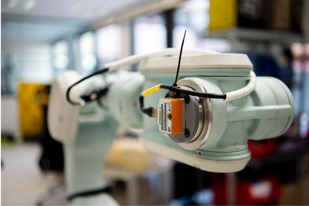
FIGURE 4.5: Picture of the IMU mounted on the PA10 robotic arm during the experiment performed to evaluate the bench true biases.
