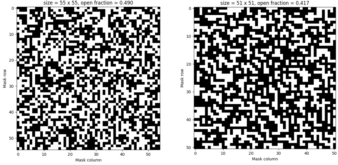
(a) Previous pseudo-random mask pattern. (b) Updated self-supporting mask pattern.
