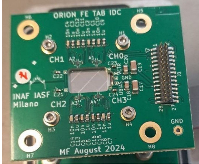
Figure 2.16. SDD front-end assembly used in the XGIS prototype activity. The SDD matrix is coupled to the front-end readout chain in order to minimize the input capacitance and preserve low-noise performance.
