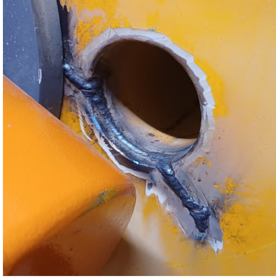
Figure 3.2: Crack repair example with full-penetration weld
