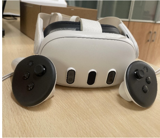
Figure 4.8: Meta Quest 3 headset used for VR simulation.
