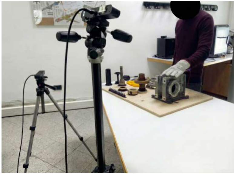
Figure 9: Example of an operator performing the Bonfiglioli reducer assembly while wearing the complete PPE configuration, with the camera system capturing the hands, tools, and assembly area from complementary viewpoints.
