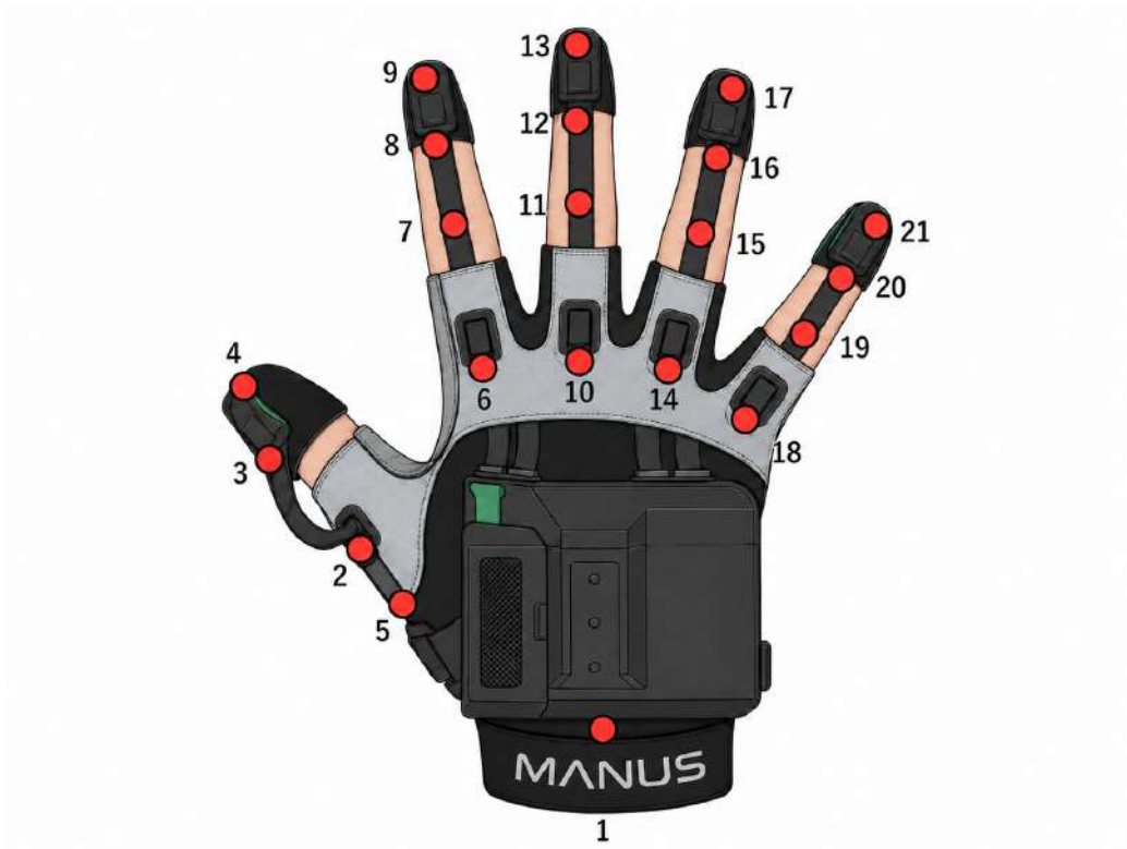
Figure 6: Instrumented hand representation used in the acquisition pipeline, showing the glove configuration and the 21 hand landmarks used for ground-truth generation and model training.
