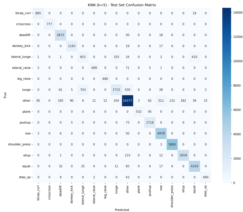
Figure A.3: KNN ( k=5 ) confusion matrix on the combined test set (91.00% accuracy). Despite high aggregate accuracy, Lateral Lunge recall drops to 46.1%, foreshadowing the same confusion pattern observed in the TCN.
