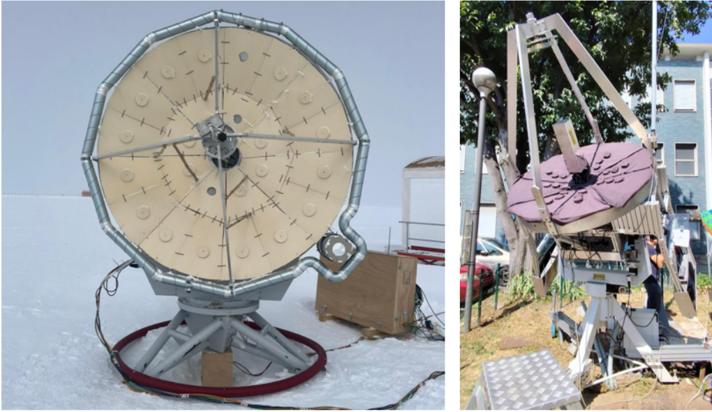
Figure 5.1: The ROSA Antenna in Concordia Station, Antarctica (Left) and the Milano Test Antenna (Right): the two Cassegrain configurations and their metallic support struts supporting the subreflector.
