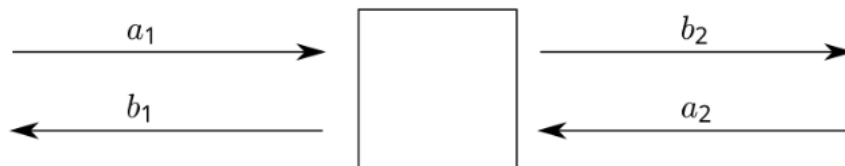
Figure 3.8: The Two-Port Network : the a vectors represent the incoming waves direction, while the b ones the exiting ones.
