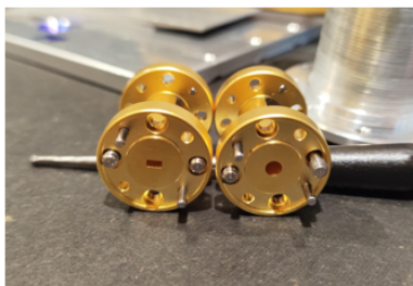
Figure 4.4: Left: the two Transition WG connected together and the view of their ends' cavities two different shapes. Right: the RF components' pair 2-Ports Network resulting S -parameters.
