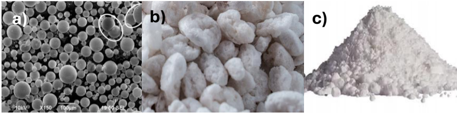
Figure 1: Photos of the materials: a) SEM photo of an assembly of microspheres [5] b) Filter perlite c) Fumed silica
