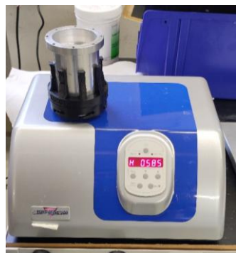
Figure 7: JEL STAV II with lower compression chamber
