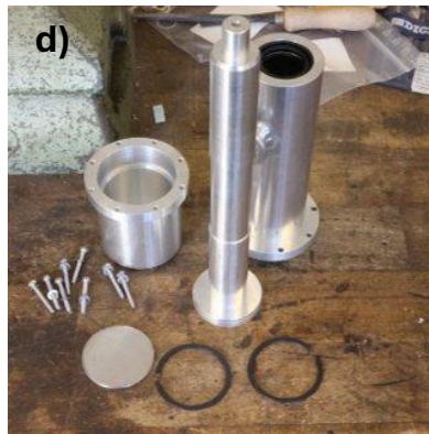
Figure 4: a) Compression with rings b) Compression without rings c) Compression chamber scheme d) General view of the components
