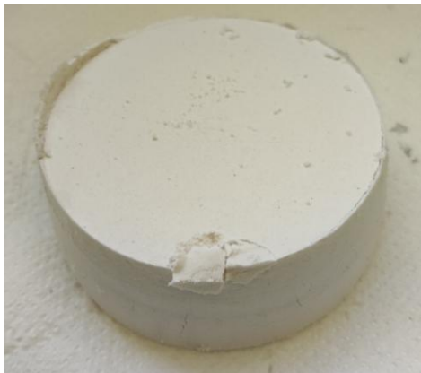
Figure 12: Example of filter perlite after compression
