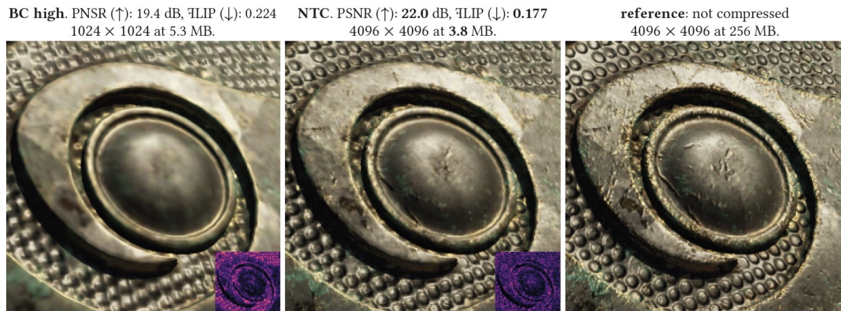
Figure 1.2: Comparison of texture fidelity with and without NTC in production environments. Source: [6]
