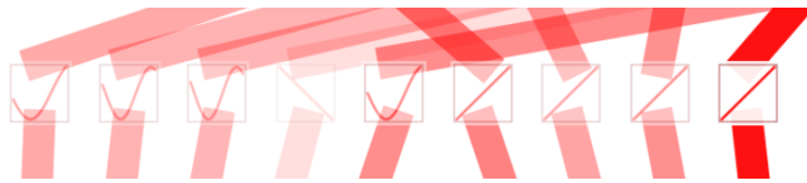
Figure 5.10: Symbolic approximation of selected input→hidden functions obtained through the KAN symbolification procedure for the 1 s model. Each panel corresponds to a learned transformation between an input feature and a hidden neuron.
