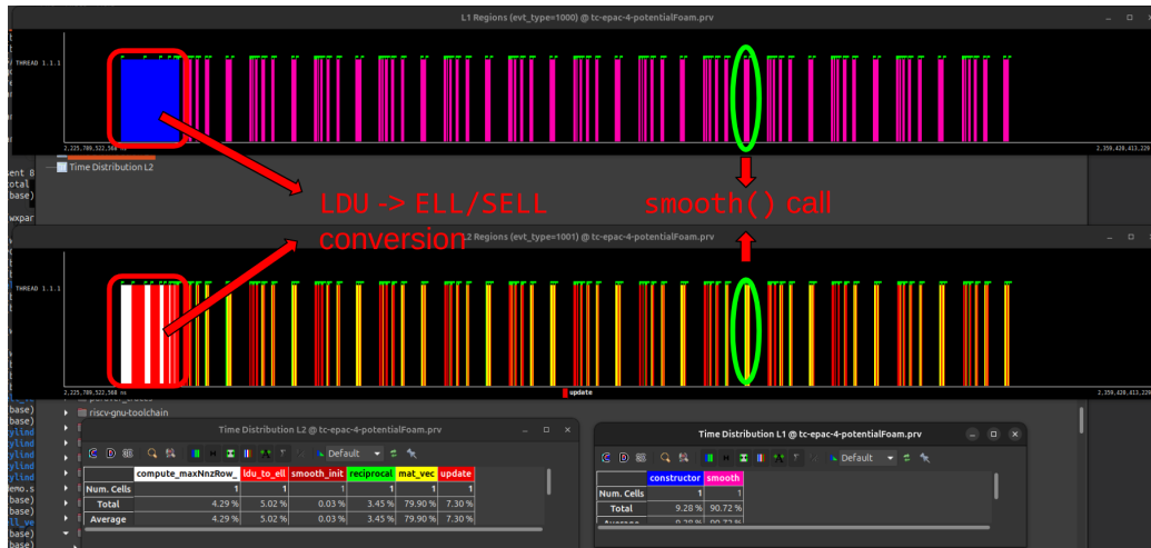
Figure 5.4: Paraver execution trace showing the time distribution of the GAMG solver phases. The setup phase overhead is safely amortized over the repeated smoother executions.
