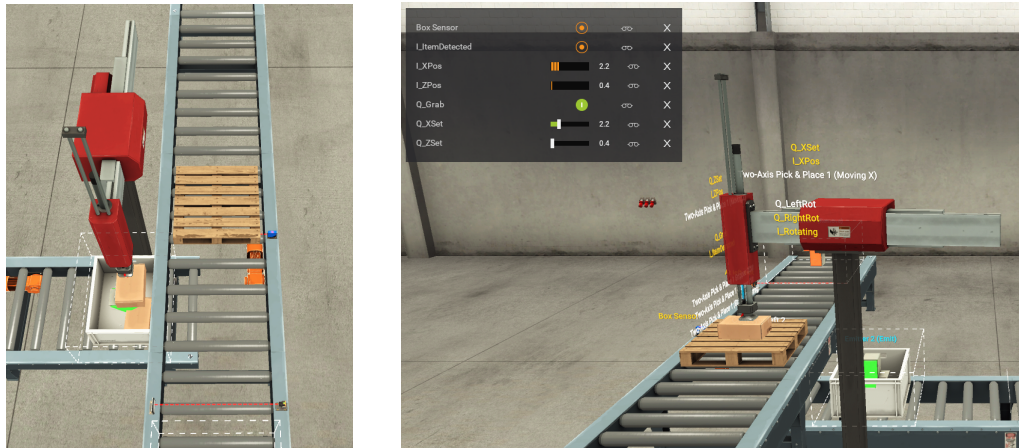
Figure 4.13: Detailed view of the Pick&Place unit during the manipulation phase of the first industrial process [4]
