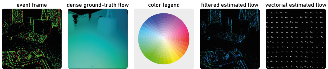
Figure 3.2.: Optical flow visualization: gradient-based and vector-based approaches
