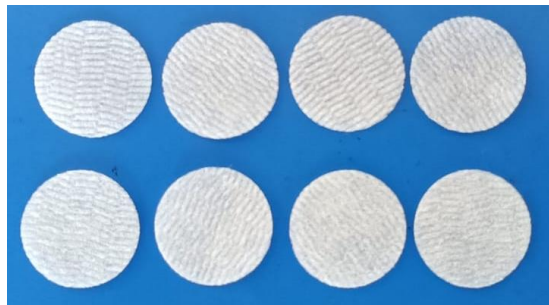
Figure 3.2 Circular melt-blown PP nonwoven samples (radius 25 mm) used in the DoEs: as-received 50/50 PP-A/PP-B fibres (bottom row) and H_3PO_4 -treated fibres (top row).
