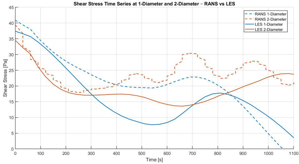
Figure 14: Shear stress time series at 1-Diameter and 2-Diameter for RANS and LES simulations.
