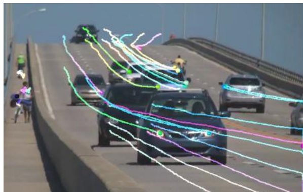
Figure 1-5 Optical flow by using OpenCV
