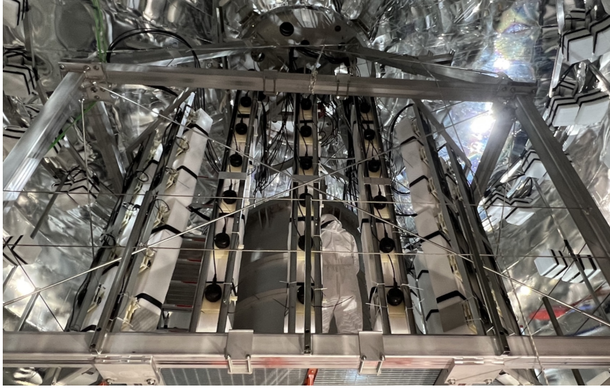
Figure 24: The Neutron Veto structure and its PMT columns situated in their final position. The ePTFE reflective panels are not present and the PMTs are protected with polystyrene foam blocks.
