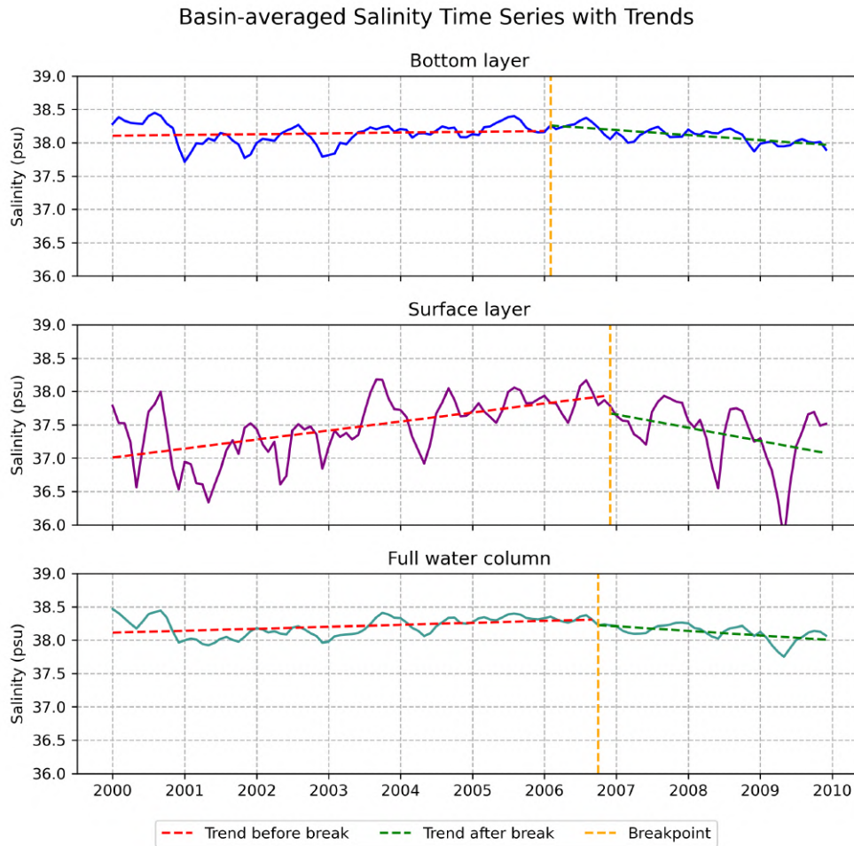
Figure 7.109: Salinity timeseries for all 3 layering methods. From top to bottom: bottom layer (blue); surface layer (purple) and full water column (indigo). The breakpoint is identified as an orange dashed line while trend before and after such breakpoint are shown in red (before) and green (after).
