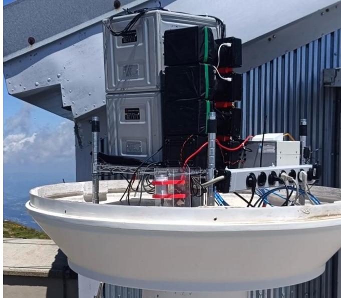
Figure 3.6: Gamma Flash current setup installed at Osservatorio Climatico “Ottavio Vittori” on Mt. Cimone. Four gamma ray detectors are inside the grey metal box on the left. On one side of this box, there is also the PC. The other four gamma ray detectors with another configuration are the black ones on the right. The weather station is shown on the back of the setup.
