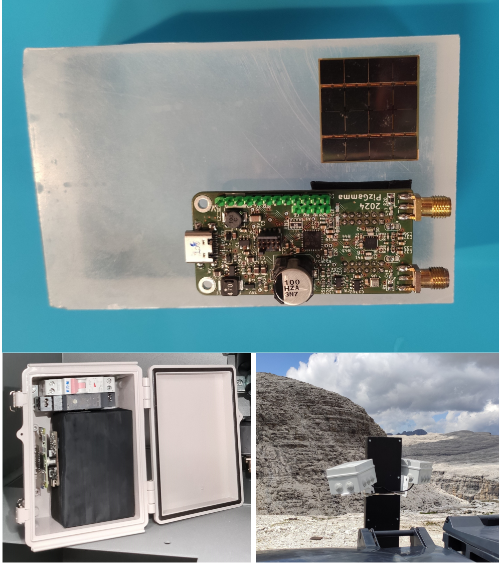
Figure 3.8: Top image : The components of one PIZ-Gamma detectors described in Subsec. 3.3.2, specifically, the scintillator crystal, the SiPM and the acquisition board are shown. Bottom image, from left to right : One of the two gamma-ray detectors of the PIZ-Gamma setup, which is placed in a sealed box. The two PIZ-Gamma detectors installed outside the Piz Boè refuge.
