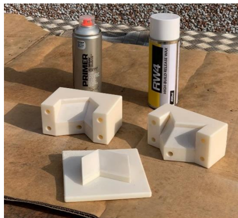
Figure 46 Mold pieces after being sprayed with primer and release wax.
