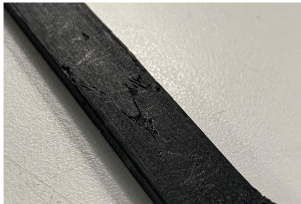
Figure 71 Fracture in the tensile specimen.
