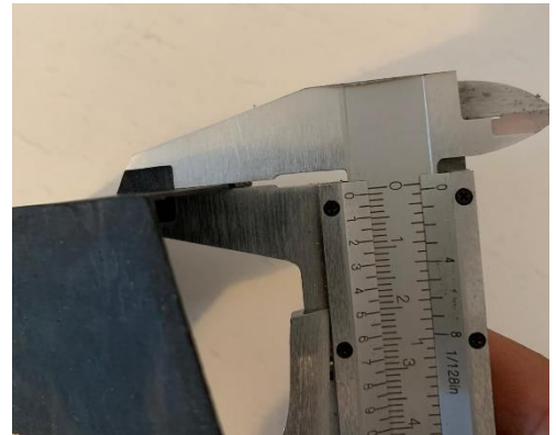
Figure 57 Thickness measurement using a Vernier caliper.
