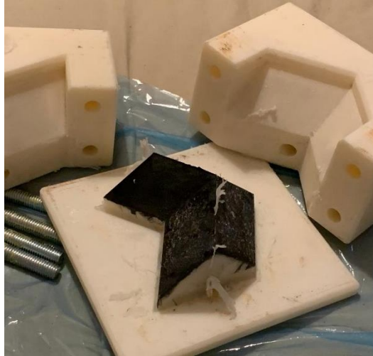
Figure 18 Open mold that requires post processing.
