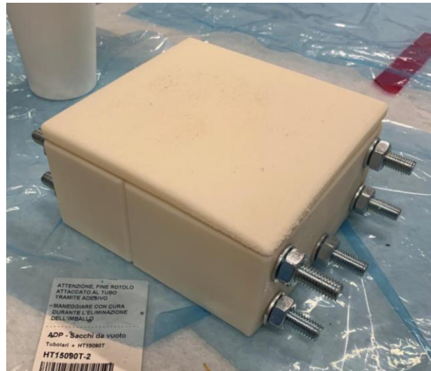
Figure 17 Closed mold compressing the fiber.
