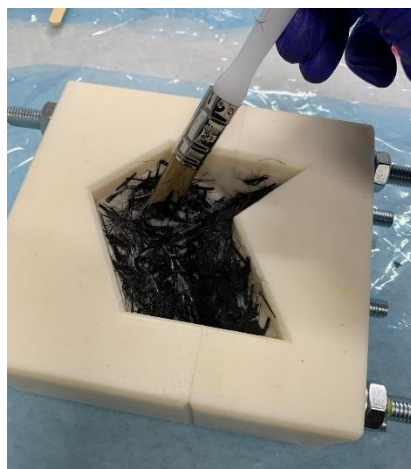
Figure 16 Impregnating short carbon fiber with resin in a mold.
