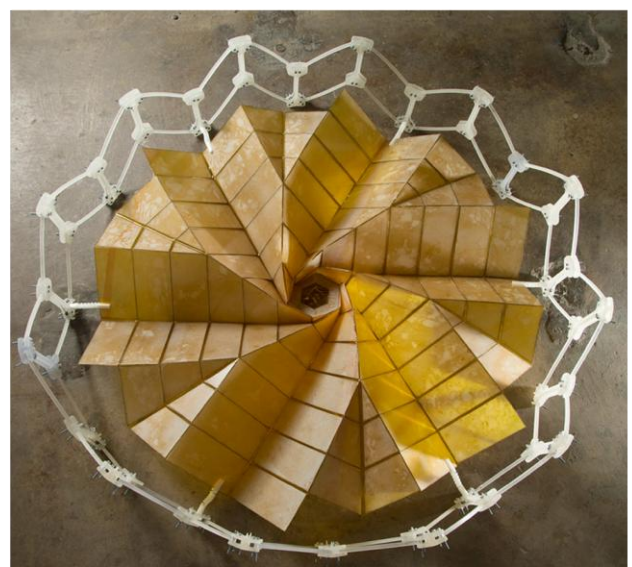
Origami-inspired solar array with a motor-driven perimeter truss
