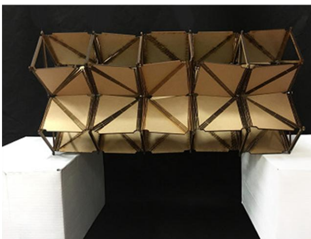
Solid reaction in Vertical force, Flexible in horizontal forces
