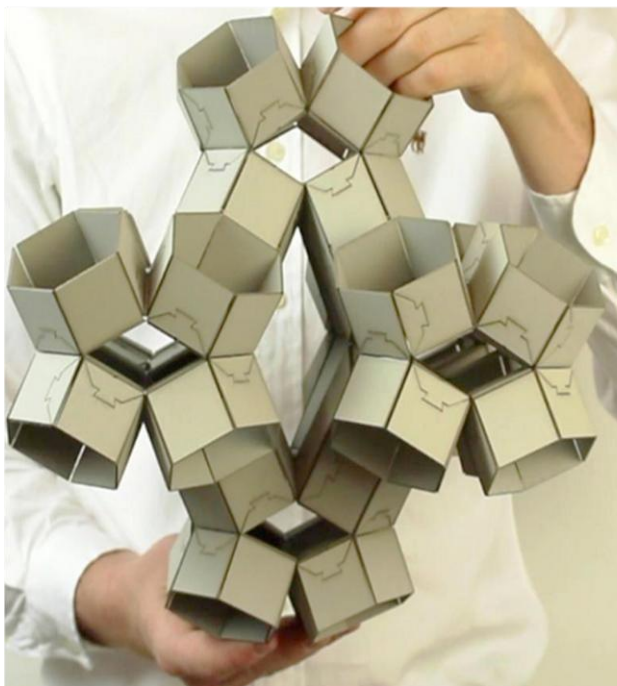
Fabrication and deformation of a single extruded cube unit cell and the corresponding mechanical metamaterial.
