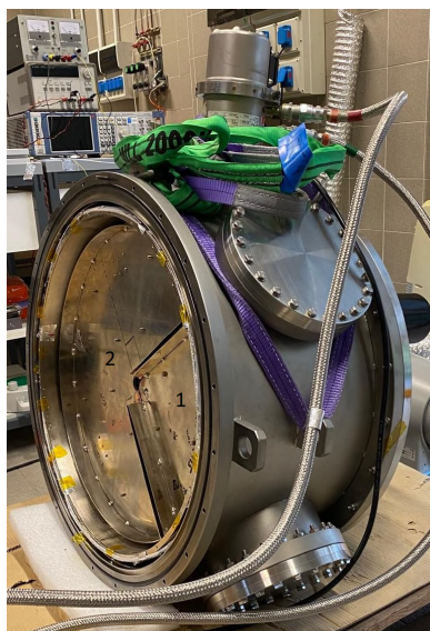
Figure 3.3: Photograph showing the external walls of the calibrator cryostat and the \frac{1}{4} and \frac{3}{4} slices, labelled respectively as 1 and 2.
