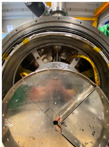
Figure 4.21: The photograph shows the slices demounted from the rotative wheel. The Si diode thermometer has been passed from the interior towards the exterior through the hole and, then, attached to the IR filter.
