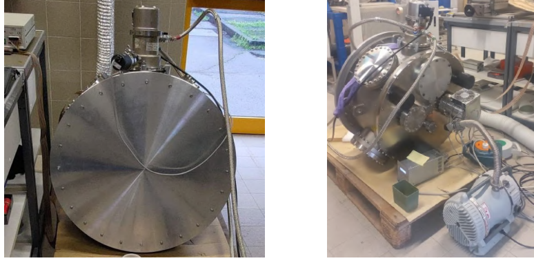
Figure 4.4: Left panel : Photograph taken at the Cryowaves Laboratory, showing the experimental setup of the first run. The Al plate in front of the calibrator cryostat is visible. The termometers deployed in the cryostat are connected to the monitor by the flat cables on the left. The flex lines are visible on the right, connecting the cryocooler cold head to its compressor. Right panel : Rear view of the cryostat, with the Scroll vacuum pump connected to the instrument through a Tombac line, by the valve of the turbo molecular pump, visible in the photograph too.
