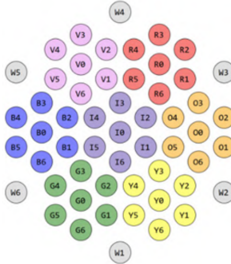
Figure 2.4: Scheme of the arrangement of the Q and W-band polarimeters in the focal plane, projected onto the sky.
