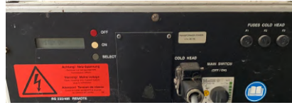
Figure A.5: Front of the compressor, connected to the cryocooler through two He flex lines.
