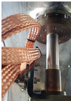
Figure 3.6: Second stage of the cold head of the cryocooler, with thermal straps.
