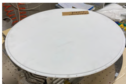
Figure 4.22: The photograph shows the IR filter before mounting it onto Strip's calibrator and attached to the thermometer.
