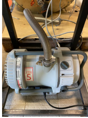
Figure A.2: The dry Scroll vacuum pump used to evacuate the calibrator (pre-vacuum).
