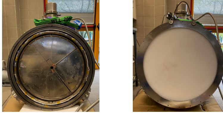
Figure 4.12: Photographs showing a front view of the calibrator cryostat. The slices, visible before the coupling with the flat (without grooves) window ( Left ) and then the UHMWPE window mounted ( Right ).
