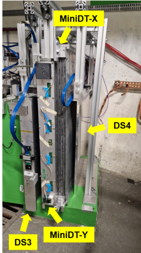
Figure 3.10: The MiniDTs and DS3-4 installed in the new mechanical support structure, as pointed by the yellow labels.
