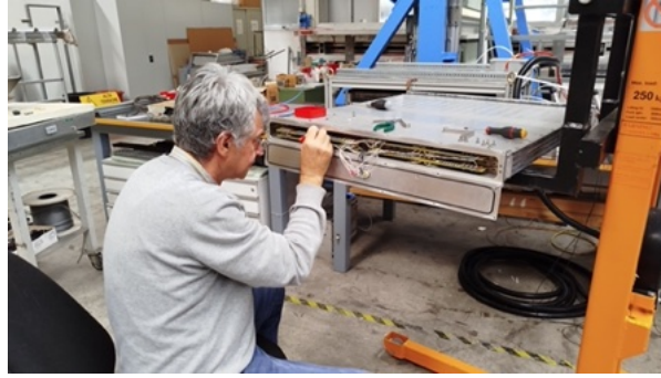
Figure 2.21: The MiniDT cathode fixing procedure.
