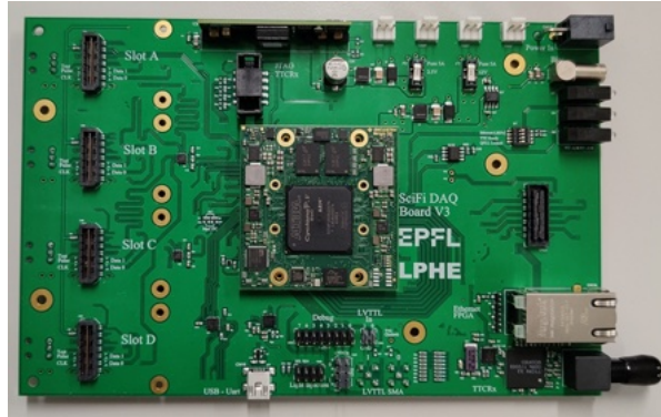
Figure 1.8: The SND@LHC DAQ board. The four FE board connectors are visible on the left, the TTCrx and optical receiver on the bottom-right [1].
