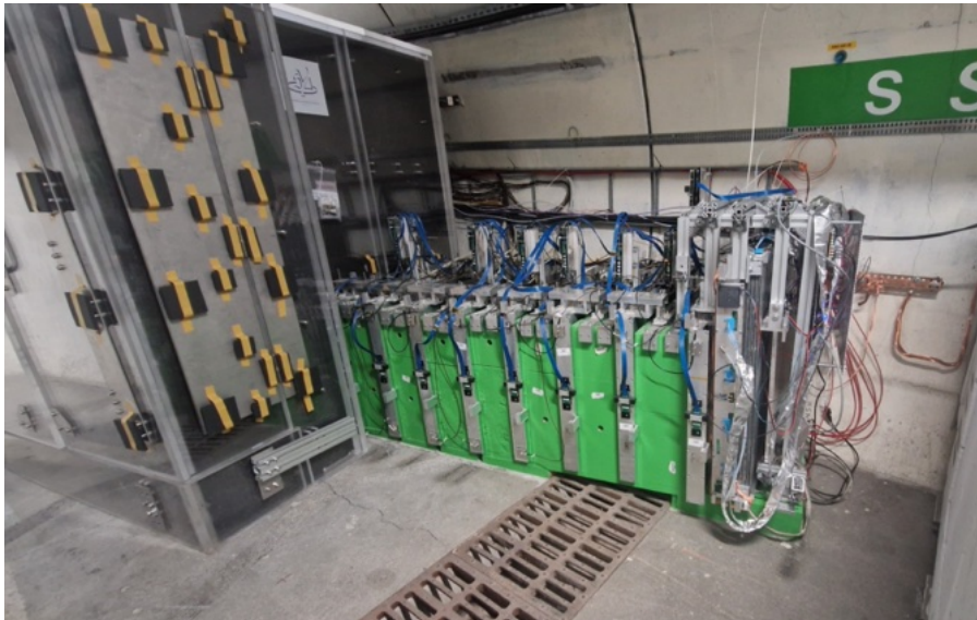
Figure 3.11: The SND@LHC experiment, with the installed MiniDTs system.
