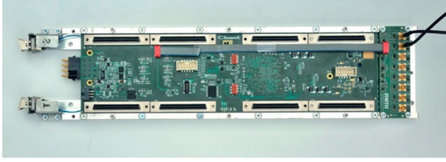
Figure 2.10: Image of the final OBDT-theta board assembled in its mechanical structure together with the OBDT-theta testpulse board [18].
