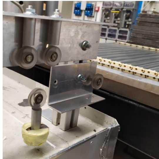
Figure 2.5: Tool used to tension the wires during the MiniDTs' assembly [17] .
