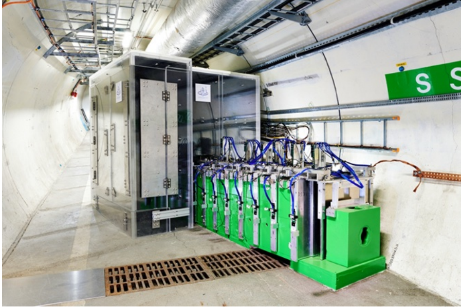
Figure 1.1: Global view of the SND@LHC detector in TI18, with the neutron shield box surrounding the target section [7].
