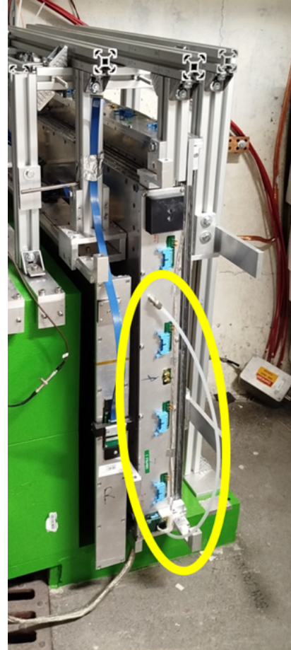
Figure 3.15: Circled in yellow, the gas link between the two MiniDTs: the gas mixture flows from the tunnel-side of MiniDT Y to the floor-side of MiniDT X.
