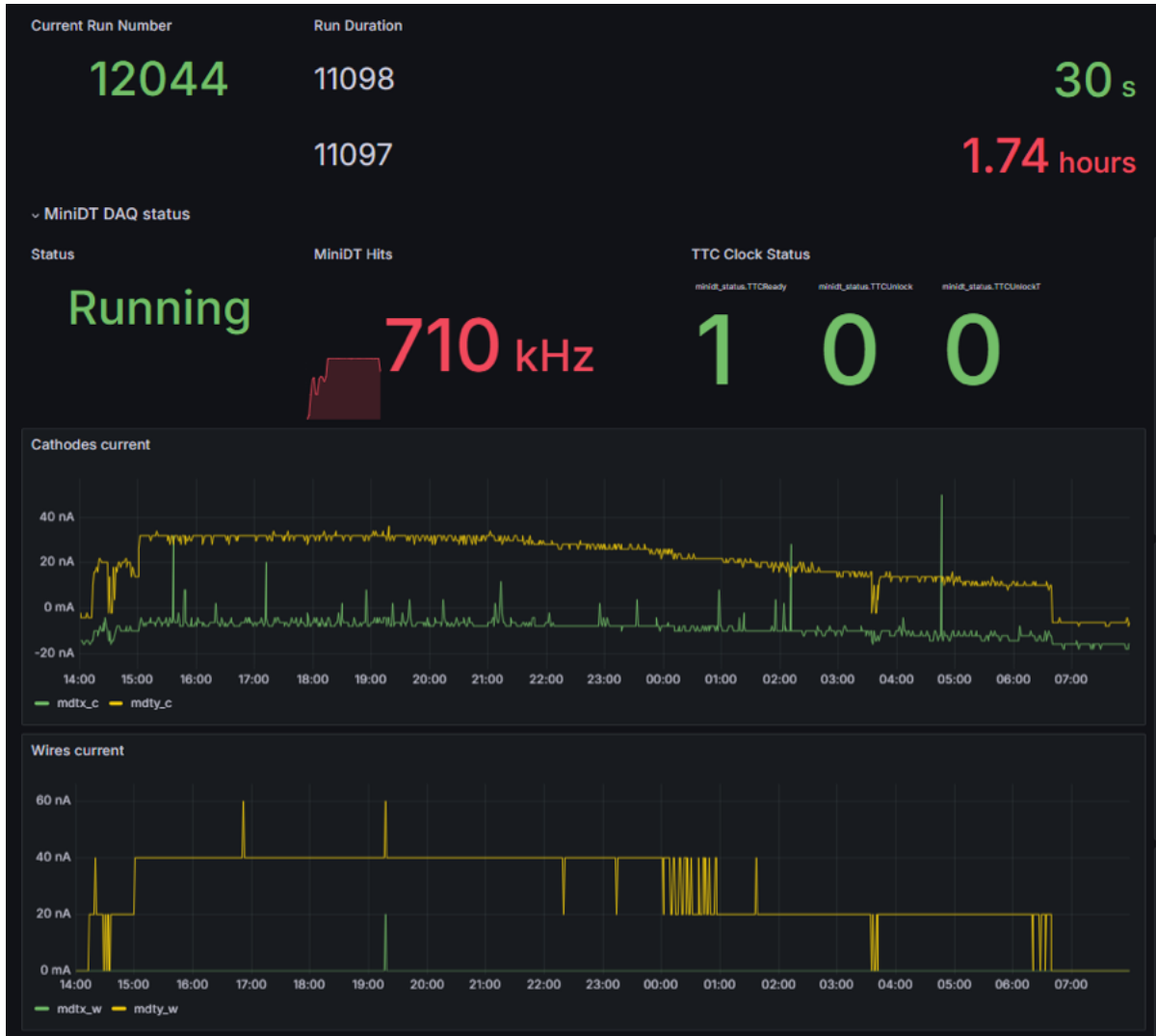
Figure 3.21: The Grafana [33] online web page for MiniDTs, during a run with colliding bunches in LHC. In the web page, a monitor comprehensive of the currents associated to the MiniDT cathodes and wires, the run status, TTCReady, TTCUnlock, TTCUnlockT signals, and TPGs and hits rates is provided.
