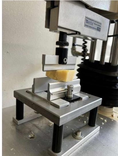
**Figura 17-** Three point bending test.
