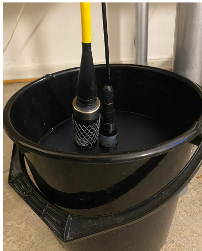
Figure 5.1.1: Test container setup with integrated sensors
