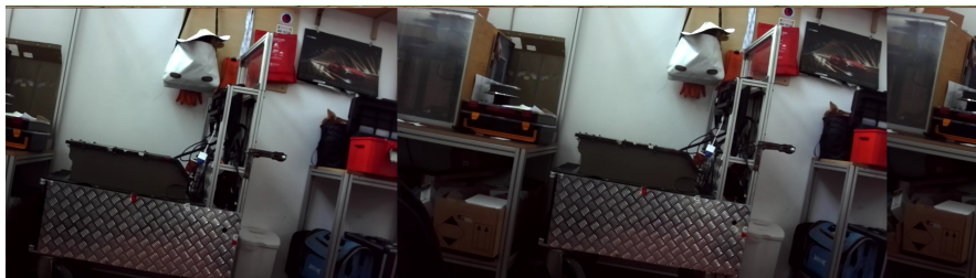
Figure 5.6: Example of a corrupted output from the camera driver. Instead of a single, sharp discontinuity at the center, multiple misaligned seams are present.
