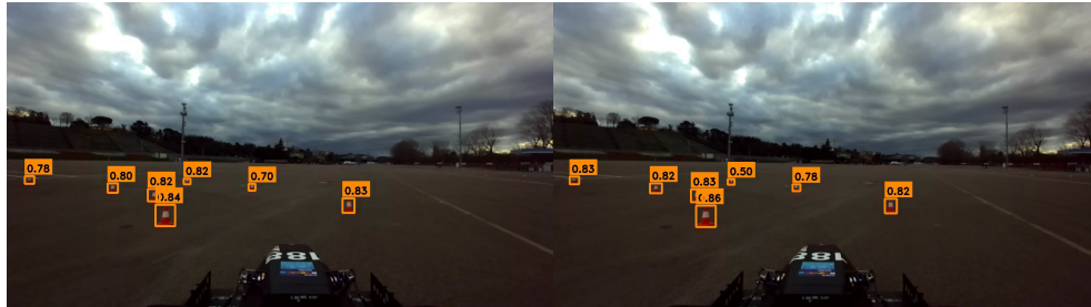
Figure 5.7: YOLO output after NMS. The numbers represent the confidence (or probability) of the detections.
