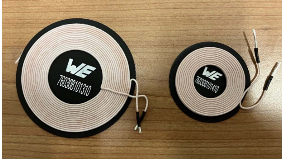
Figure 4.7: Photo of the receiver (on the left) and the transmitter (on the right) coils. Image retrieved from [50].
