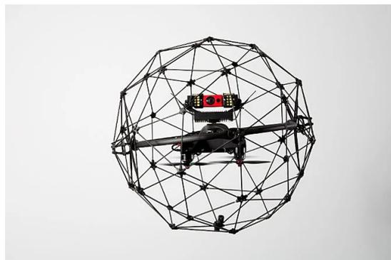
Figura 1.4: Decouple Cage
