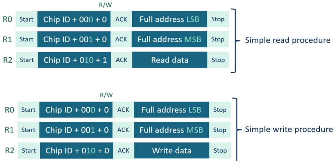
Figure 3.3: Simple Read/Write procedures for LIROC I2C slow control and configuration.
