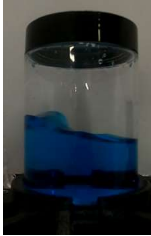
Figure 5.22: Instant peak of the liquid, container IC at the end of Trajectory Volumes 2 with \bar{\eta}_{lim} = 25 mm.
