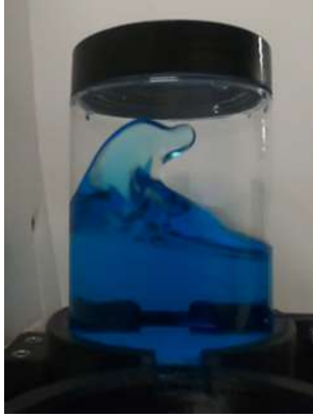
Figure 5.17: Instant peak of the liquid: third regime of motion; EC container during optimized motion-law with t_{end} = 3.76 s.
