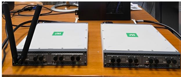
Figure 4: Two NI Ettus USRP X410 devices used in the O-RAN setup
