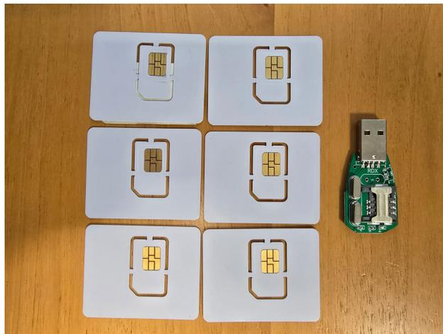
Figure 6: Open Cells SIM cards and SIM card reader/writer
