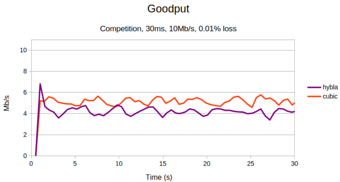
Figure 4.27: First 30 s of a connection that lasted 300 s, Competition between Hybla and Cubic, RTT: 30 ms, bandwidth 10 Mb/s, 0.01 % loss
