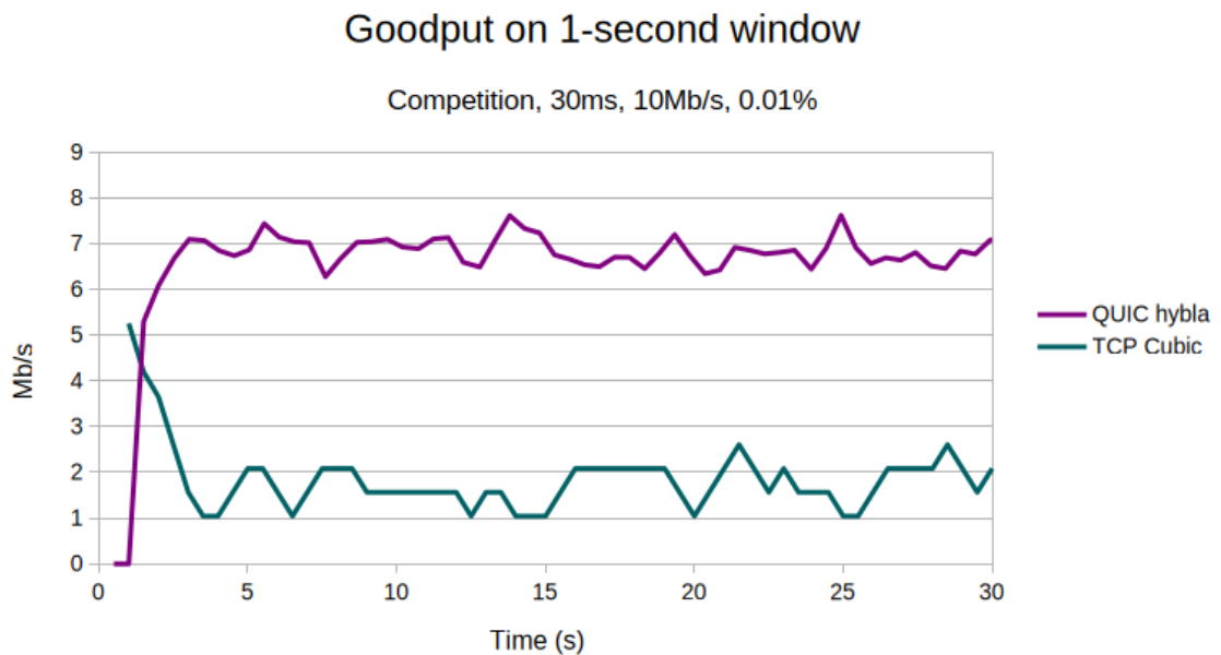
Figure 4.36: First 30 s of a connection that lasted 300 s, Competition between QUIC Hybla and TCP Cubic, RTT: 30 ms, bandwidth: 10 Mb/s, 0.01 % loss
