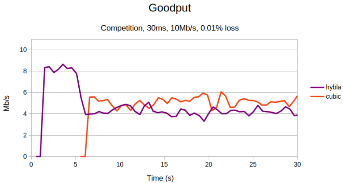
Figure 4.29: First 30 s of a connection that lasted 300 s, Competition between Hybla and Cubic (started 5 s after), RTT: 30 ms, bandwidth 10 Mb/s, 0.01 % loss
