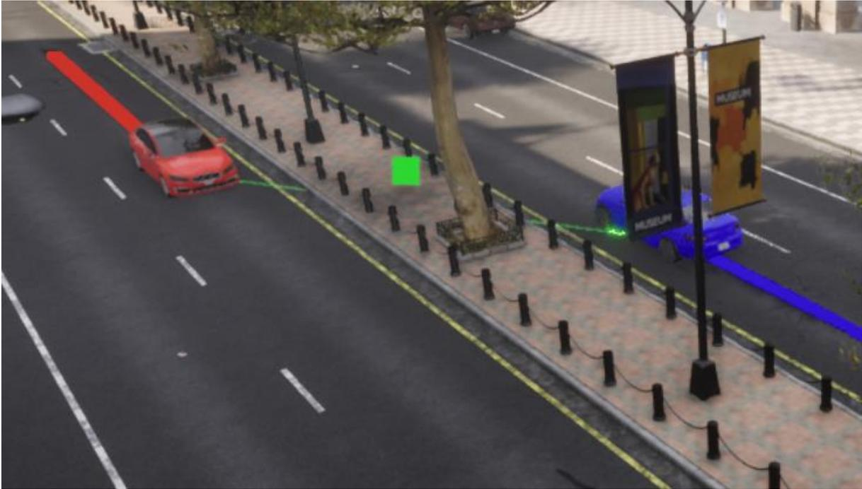
**Figure 25: Rendezvous detection in Scenario 1. Green lines represent the LIDAR data exchange between the vehicles and green dot is the rendezvous point**
