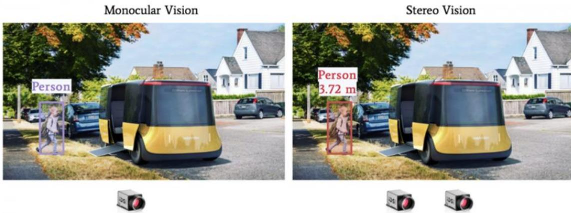
**Figure 6: Monocular vision vs. Stereo Vision [9]**
